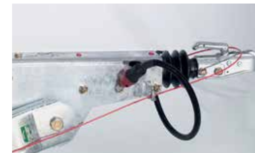
Ball trailer coupling for height-adjustable drawbar
