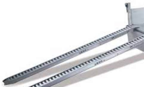
Aluminium ramps (up to 1.9 load capacity / length 2465 mm; up to 2.3 t load capacity / length 2230 mm; up to 2.8 t load capacity / length 2650 mm)
