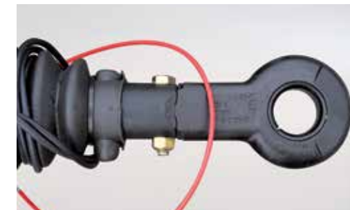
DIN towing eye for height-adjustable drawbar
