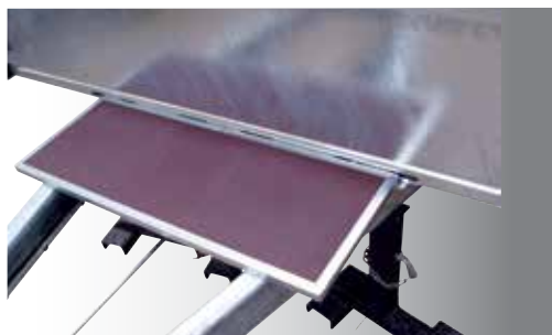
Excavator bucket support for V-shaped draw bar
