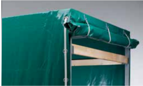
Tarpaulin and frame, load height 1300 mm / 1600 mm / 1800 mm / 2000 mm
